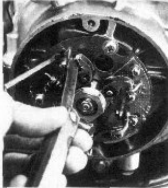
4. Both sets of points should be adjusted between .012 and .016. This is fairly critical, so work carefully and be sure the setting is within the indicated tolerance.
