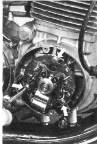
7. By loosening these three screws (arrow) the entire base plate can be turned, thereby enabling the tuner to time cylinders one and four at full advance.
