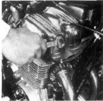
1. Using a 17 mm wrench, remove all of the valve adjusting caps.
