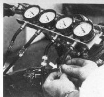
21. Adjust each gauge so it reads between 8 and 9 lbs. psi. Take all the flutter out with the bleeder valve with no more than 1 lb. of needle bounce. These gauges sell for about $10 each.
