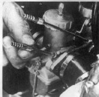
16. Remove the threaded plug in each carburetor and insert a C100 (Honda) main jet with a short tube soldered to it.
