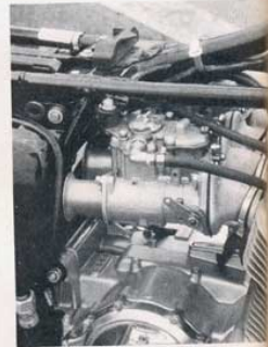
This picture clearly shows installation and mounting of the carburetors. There is just enough room between the velocity stacks and the frame to fit an air cleaner.
