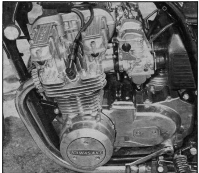
The compact KZ650 engine features DOHC valve actuation and a Hy-Vo primary chain. The cylinder head and block casting have cooling air passages to direct air over combustion chambers and between cylinders.
