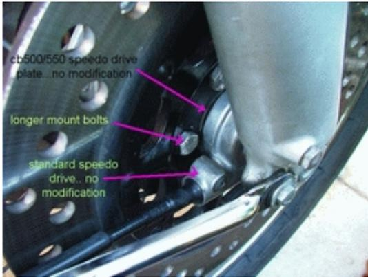
Now put the CB500/550 speedo drive plate in the middle of the second disc, it should be a really neat [tight] fit, but it should fit, you won't be able to use your chrome dress ring - no room. Next put your speedo gearbox on, then refit your axle. If you have forgotten which side the shaft goes into, it insets from the speedo side, once this is done, your front double disc wheel is complete. Now the caliper.
