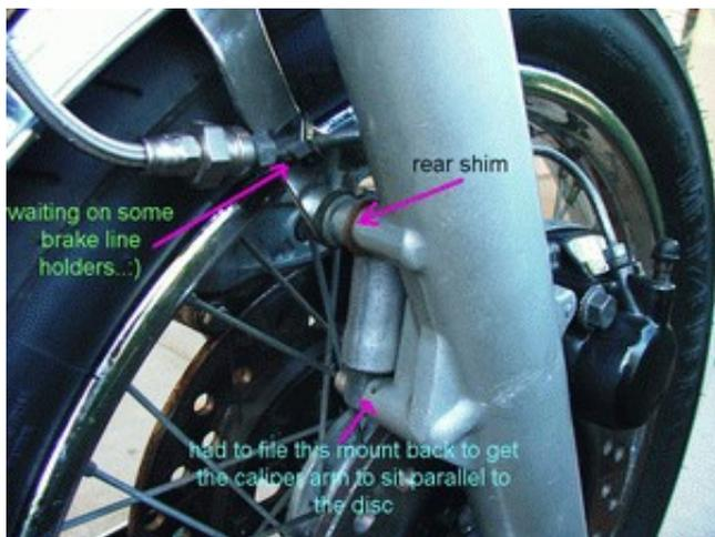
This took some time to get right, because you have to file the pivot mount parallel to the disc as well, otherwise the top of the pivot arm won't mount to the fork. Take your time; you can always take metal off - its bloody hard to put it back on though, and also remember that there are metal filings going into the threads - blow these out before screwing a bolt into them otherwise it will destroy the thread, and that's not a good thing.
