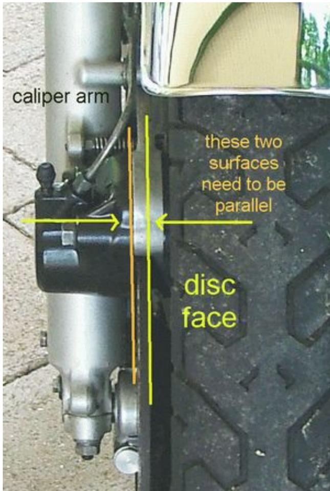
Now what I did was try and file the lower mount as close as I could to the fork leg, without fouling up the pivot arm, before I started shimming the top of the mount. (fig. 3)
