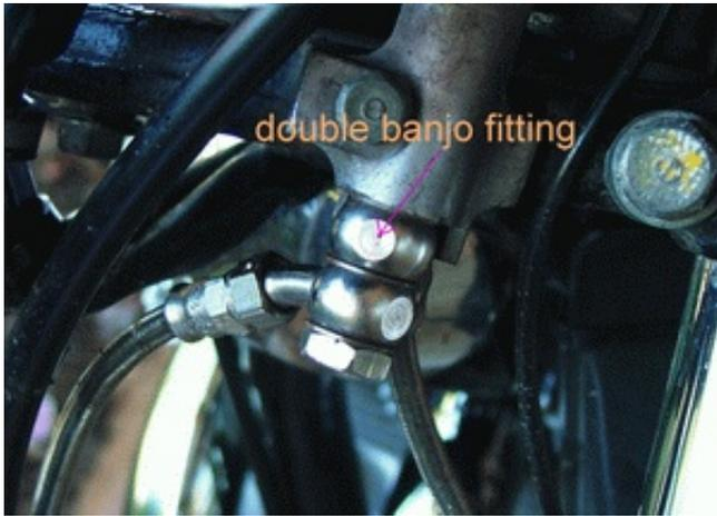
You will notice that I am using stainless braided lines. I got my local hydraulics shop to make them for me, but the standard factory lines will fit as well. Connect your steel line (fig4) to your new lower line and this part of the conversion is done.
