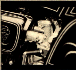
Stock carburetors use alloy air horns for breathing.
